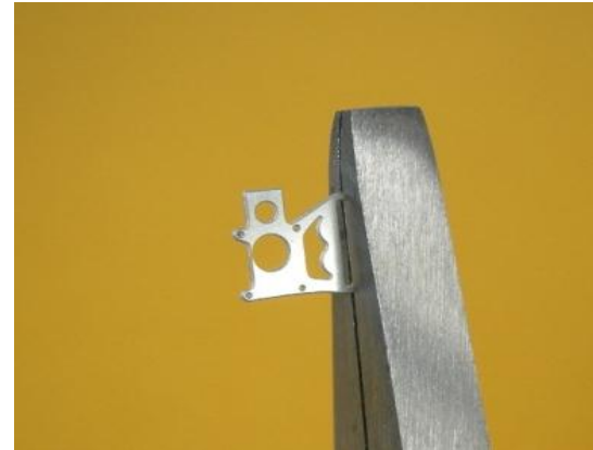
After bend, fit slot over rotor and bend 90-degrees
