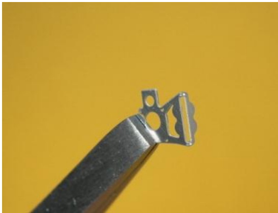
Example of bracket after 90-degree bend
