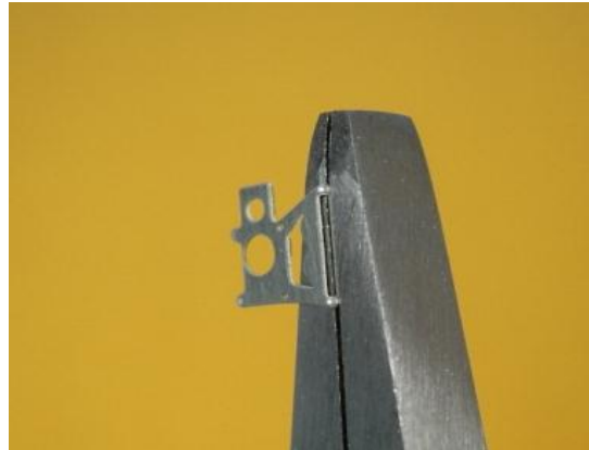
Grasp bracket so edge of pliers are flush with outer edge of rotor slot
